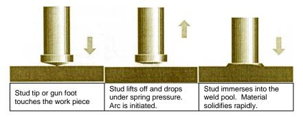
Note the final picture above; for the weld to be good, it should have an even fillet completely around it. Any voids, at all, indicate a weakness in the weld zone that could cause weld failure later. Also, the stud should appear to penetrate the parent material. It should never appear to be "sitting on top" of the weld.
