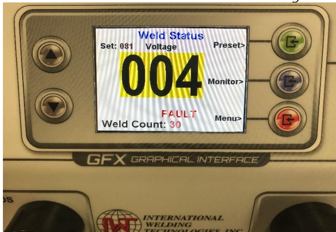
(Transformer Thermal Protection on Weld Status Screen)
