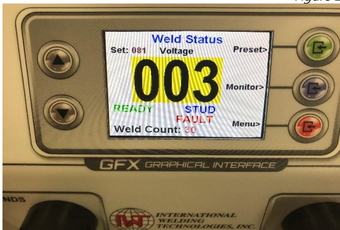
(Charge Start Fault on Weld Status Screen)
