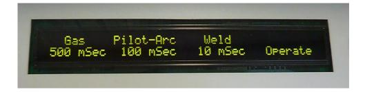
During a weld cycle, the OLED display will provide feedback in real time.
