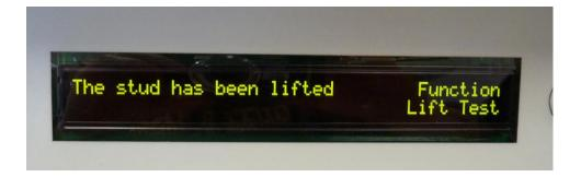
The above screen ends the lift check. **Note:** a weld cannot be made during a lift check. If the gun fails to lift the OLED display read "gun did not lift".
